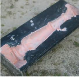
*Deris is a special release agent with dual purpose: By one side, the release agent and for another side retardant that allow the faced aggregate finish with different particle-size.*
